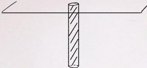
Goal: Model the displacement  $u(x)$  of the elastic bar at each position  $x$  under gravity.
